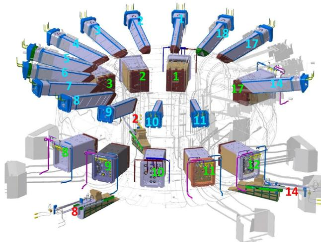
Figure 1. The ITER diagnostic port plug, divertor (3 ports, red numbers), Equatorial (9 ports, green numbers) and upper (14 ports of which 10 have significant payload, cyan numbers). For scale, the flanges of the ports are approximately 15 m from the machine vertical centerline.
