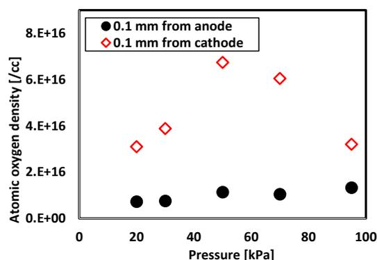
Fig. 2. Pressure effect of max O density.
