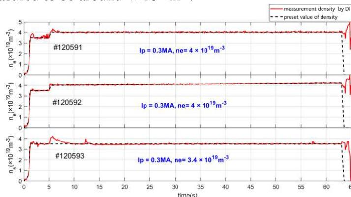
Figure 1. Good agreement between the density measurement results obtained by the DI system and the preset values of density.
