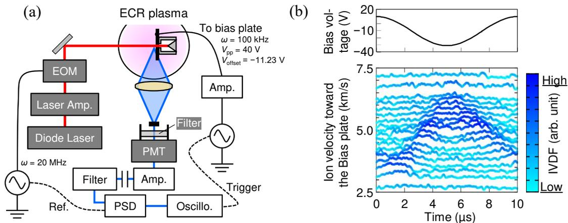
Figure 1. (a) Schematic diagram of time-resolved LIF system. (b) Temporal evolution of IVDF measured at 1 mm from the bias plate plotted with the bias-voltage waveform at 100 kHz.
