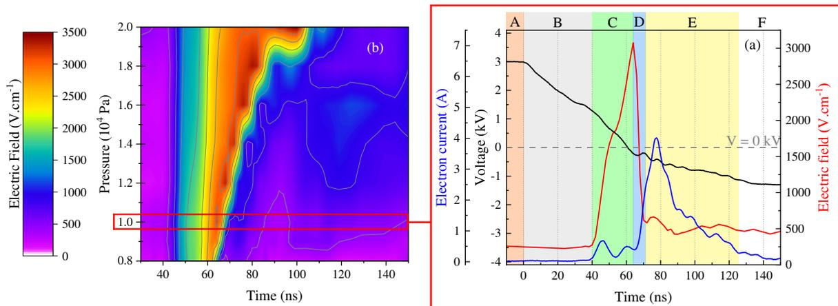
Figure 1. (a) Cartography over time and gas pressure, from  $0.8$  to  $2.0 \times 10^4$  Pa, during the positive to the negative transient polarisation of upper electrode. (b) Focus of the electric field (red curve) and electrical (black and blue curves indicating respectively applied voltage and current variations) measurements for the  $10^4$  Pa gas pressure condition. Pure ammonia, applied voltage  $6 \text{ kV}_{pp}$  and gap  $3 \text{ mm}$ .
