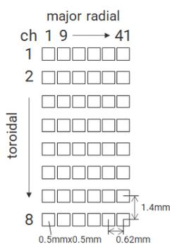
Figure 1. Layout of MCT detector for 2D-PCI
