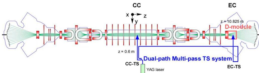
Figure 1. Schematic of GAMMA 10/PDX and DPTS.
