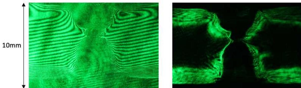
Figure 1. An example of simultaneously taken Interferogram (left) and dark-field Schlieren image (right) of the 25  $\mu\text{m}$  Cu from an X-pinch plasma.
