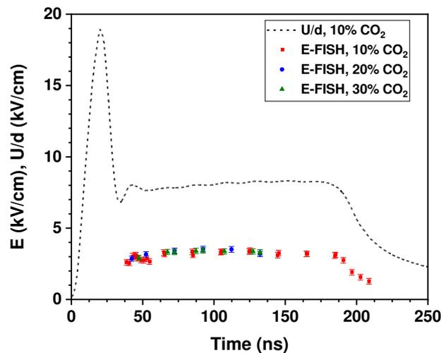
Figure 1. Electric field in ns-APPJ measured by E-FISH technique together with voltage over gap (1 mm) ratio for different N<sub>2</sub>:CO<sub>2</sub> mixtures at pressure of 150 mbar and gas temperature of 340 K.
