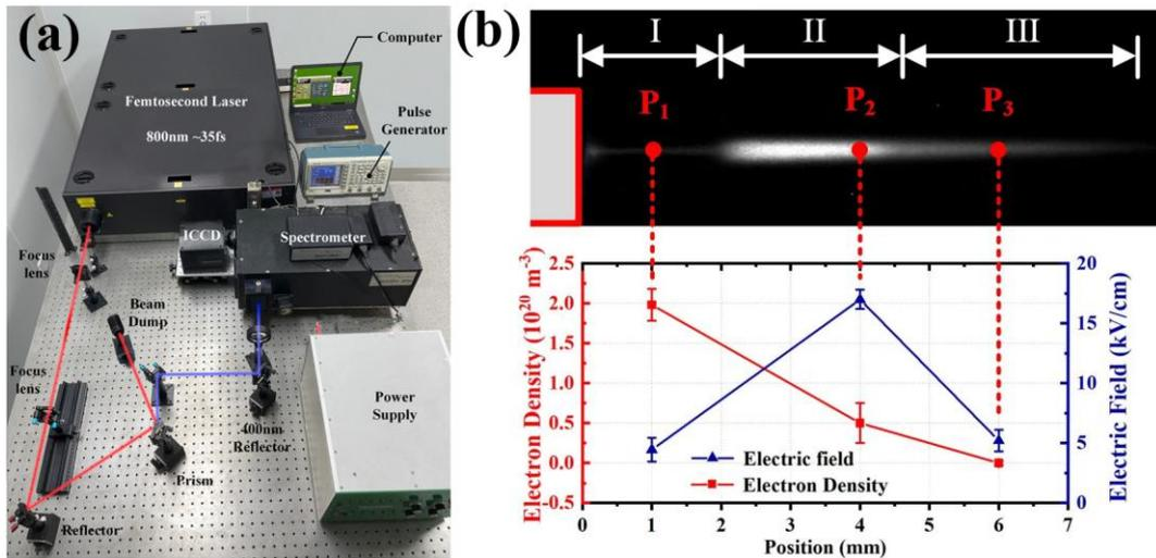
Figure 1. (a) Schematic of electric field induced second harmonic (E-FISH) system. (b) The electron density and electric field at different positions.
