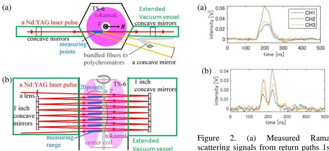
Figure 1. (a) The vertical and (b) the horizontal cross section of the experimental setup.
