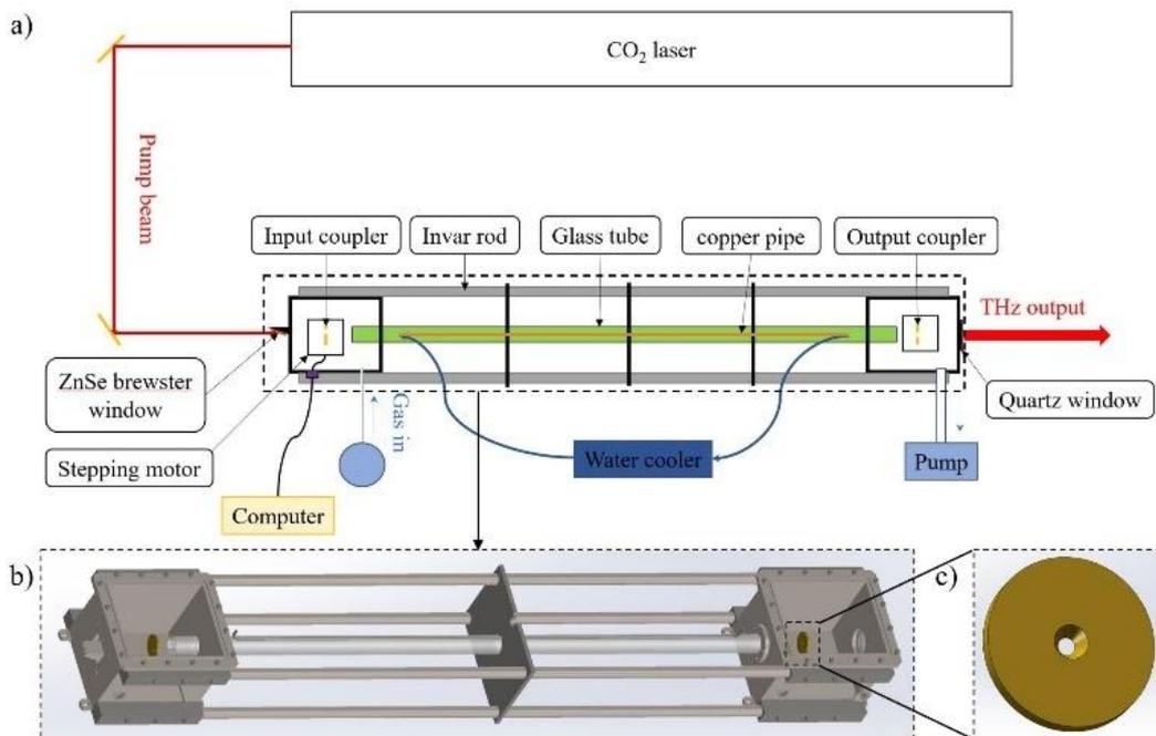
Figure 1. a) Diagram of CO<sub>2</sub> laser pumped methanol gas laser. b) Terahertz laser resonant cavity. c) Centric-hole gilded copper mirror.
