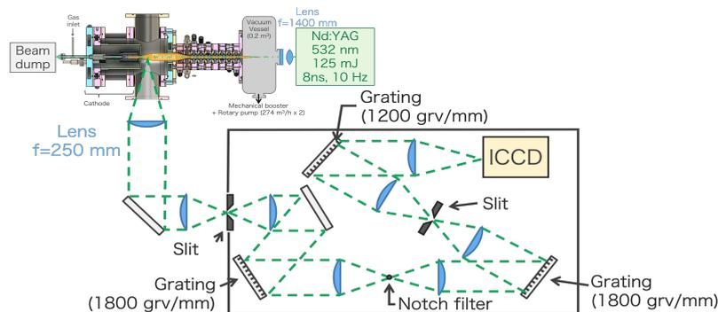
Figure 1 Schematic diagram of the cascade arc device and the Thomson scattering measurement system with a triple grating spectrometer.
