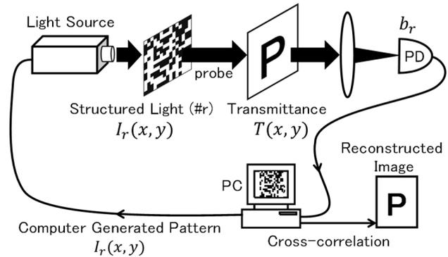
Figure 1. Schematics of ghost imaging absorption spectroscopy system.
