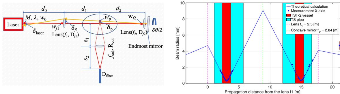
Figure 1. Schematic configuration of double-pass scheme (left), measurement and theoretical calculation of the beam radius along the double-pass optical path (right).
