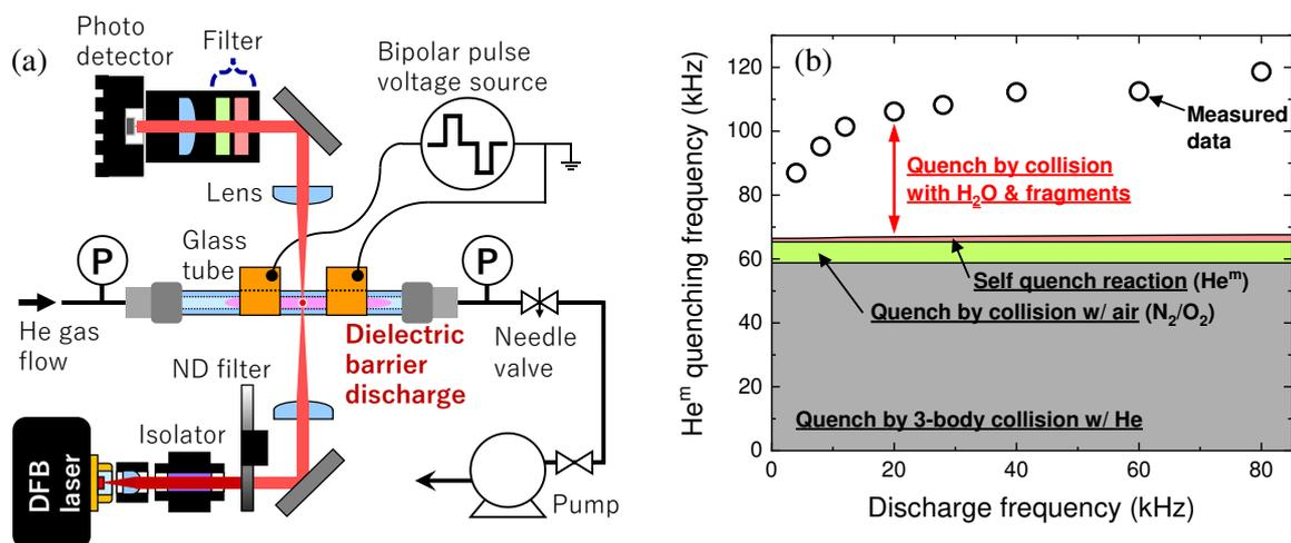
Figure 1. (a) Experimental setup of He-DBD and LAS used in this study. (b) Dependence of  $\text{He}^m$  quenching frequency on the discharge frequency measured by the LAS method. The contribution of gas species to the  $\text{He}^m$  quench is shown to investigate the influence of  $\text{H}_2\text{O}$  decomposition.
